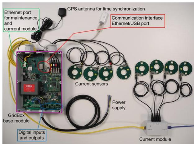
**Figure 1.** GridBox base module, current module and Rogowski sensors.
