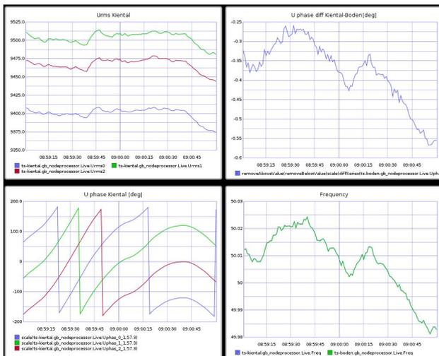
**Figure 5.** Voltage magnitude and angle, angle difference between two neighbouring transformer stations and frequency during two minutes.
